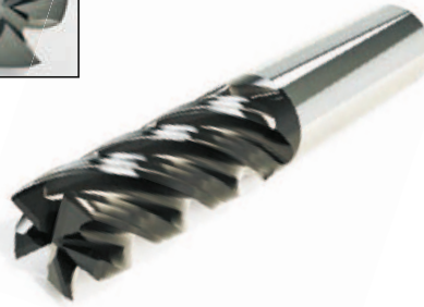
Flutes Offset for Vibration Reduction
